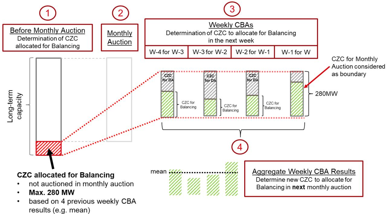
Figure 4: Process for the allocation of CZC for the balancing market
